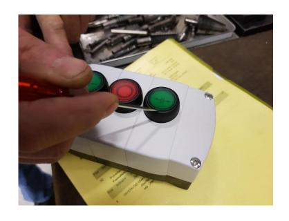
Lift the lid of the push button with a small screw driver
