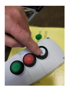
Take off the inner cap with symbol by flipping the push button station.
